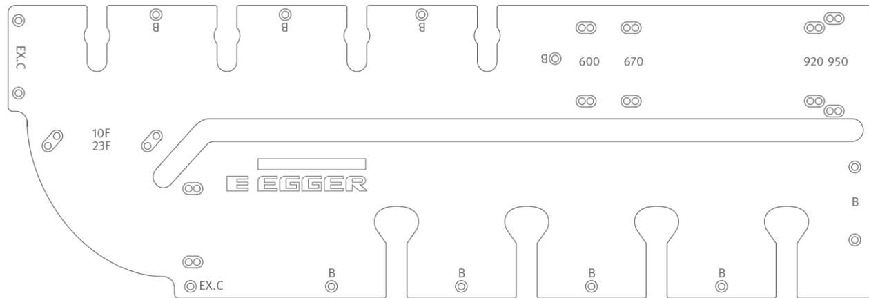
This jig can be used to fit 90° corners for all EGGER worktops. It has fixed worktop width settings of 600 mm, 670 mm and 920 mm and 950 mm. However, it can be used to cut worktops of any width smaller than the maximum capacity of the jig (950 mm) using appropriate shims and spacers.
