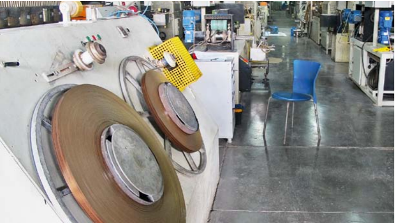
The extrusion plant handles all processes, from mixing the raw materials, printing the edging and rolling it up. Extruders play a prominent role in Roma Plastik production processes from start to finish.
