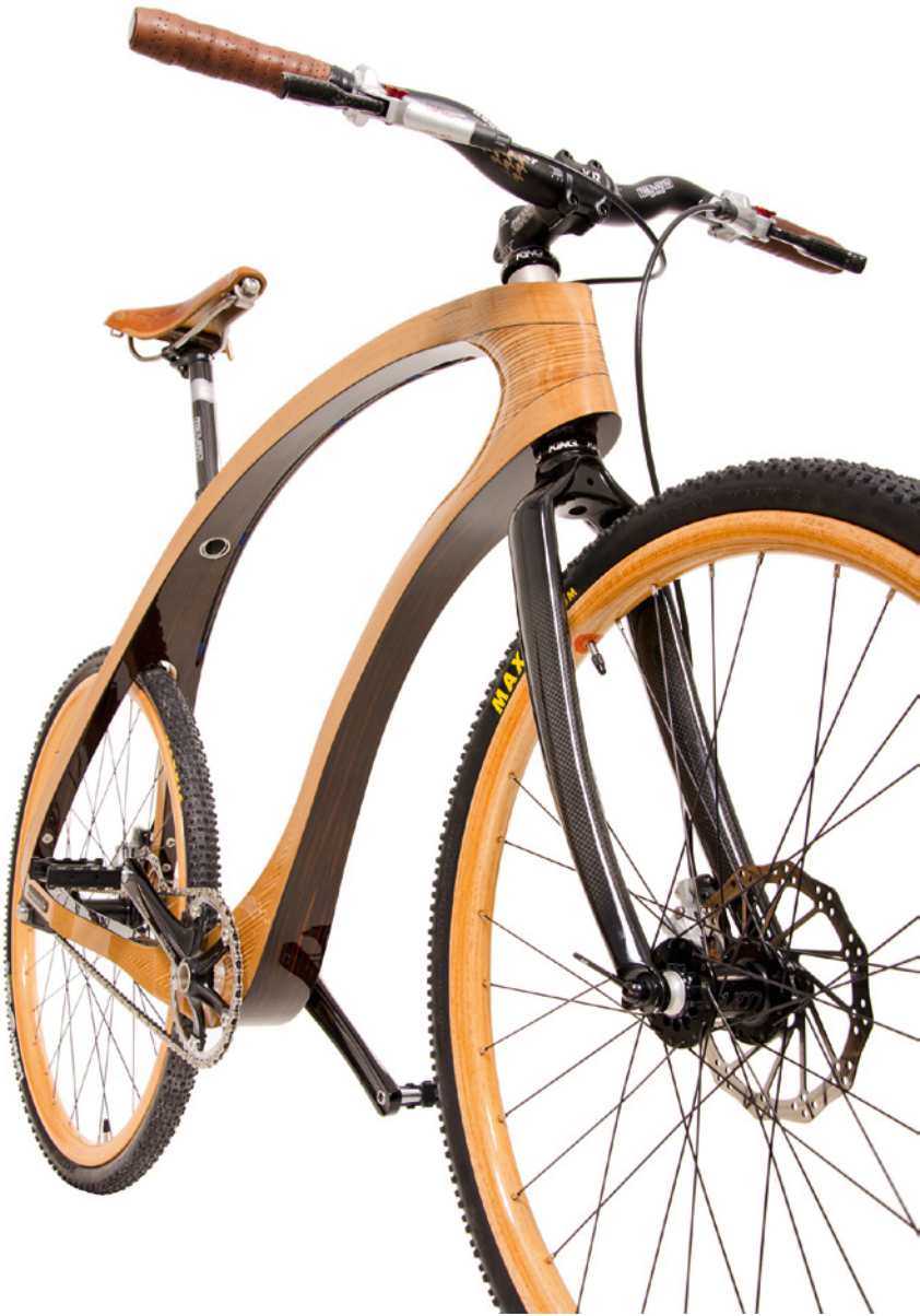
The idea behind the “Waldmeister Bike” is a wooden frame with the characteristics of a leaf spring: stability and, at the same time, flexibility. Each frame is made up of 96 0.5-millimetre layers of wood.
