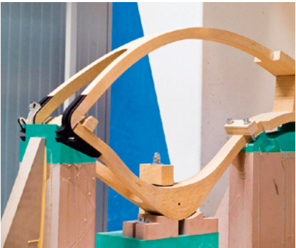
The idea behind the “Waldmeister Bike” is a wooden frame with the characteristics of a leaf spring: stability and, at the same time, flexibility. Each frame is made up of 96 0.5-millimetre layers of wood.
